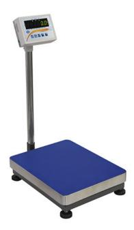
Calibratabletabletop scale / platform 400 x 500 mm or 500 x 600 mm /bi-directional RS- 232 interface / item counter / Summation function / RS-485, analogue outputs 4-20 mA, 0- 10 V optional
